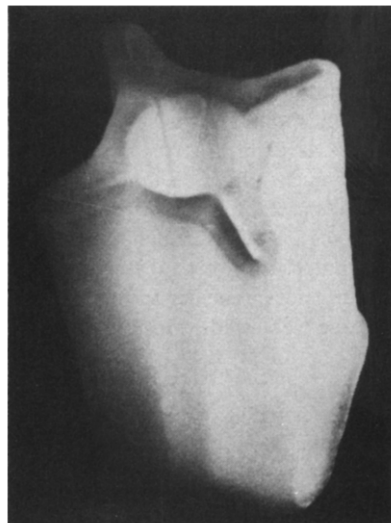
FIG. 2. Photograph of a specimen that had solidified about a finned tube.
